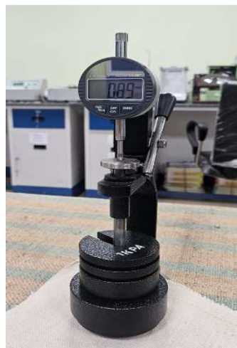
Fig. 8: Testing of percentage compression under 10 kPa
