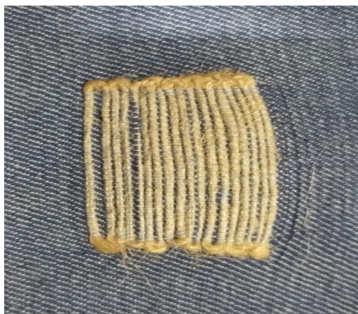
Figure 2 and Figure 3: Handloom Denim with extra weft designs using Jute and colored floating weft
