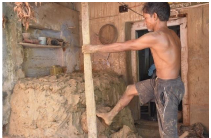
Figure 1: Clay preparation in Panchmura: kneading and tempering clay with sand and khar (dried paddy plant). Source: Author (fieldwork)
