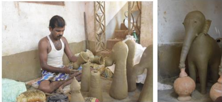
Figure 2: Forming process in Panchmura: shaping clay forms on a manually operated pottery wheel. Source: Author (fieldwork)
