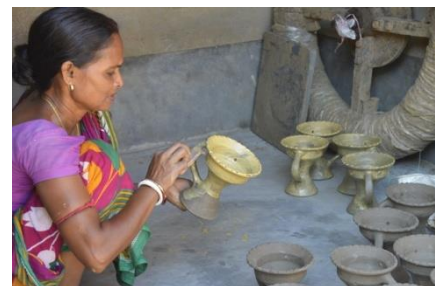
Figure 4: Preparation and application of natural clay slips (Khadigad, Banak, and Bhalogad) for surface treatment prior to firing. Source: Author (fieldwork)
