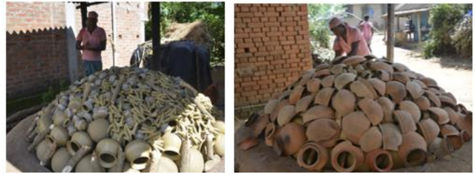
Figure 7: Preparation of the kiln for firing: placement of wooden fuel and covering of the kiln top with broken terracotta shards to form a dome structure. Source: Author (fieldwork).
