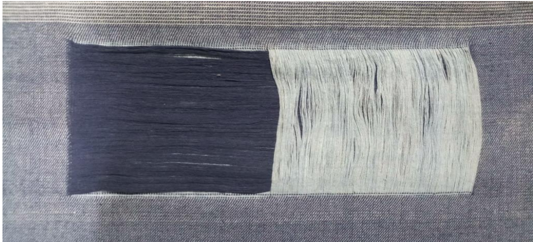
Figure 4: Handloom Woven Denim with extra weft using cotton yarn
