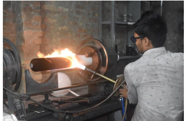
Figure 1: Hollow glass tube forming process
