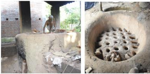
Figure 6: Traditional kiln structure in Panchmura, showing the cylindrical form, fire chamber, and upper loading chamber used for firing terracotta artifacts. Source: Author (fieldwork)
