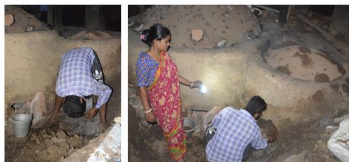
Figure 8: Reduction firing process: addition of cow dung cakes and sealing of the kiln to create a low-oxygen environment for black surface formation. Source: Author (fieldwork).
