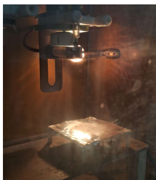
Fig. 2: Nanofibre mat formation in the electro spinning machine
