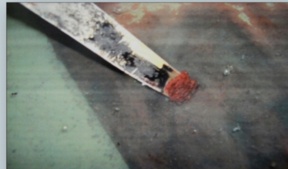
Deposition of Copper sediment on the plate
