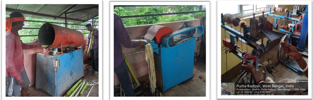
Fig. 1. Cutting of the banana stem, extraction of fibres and conversion into yarn
